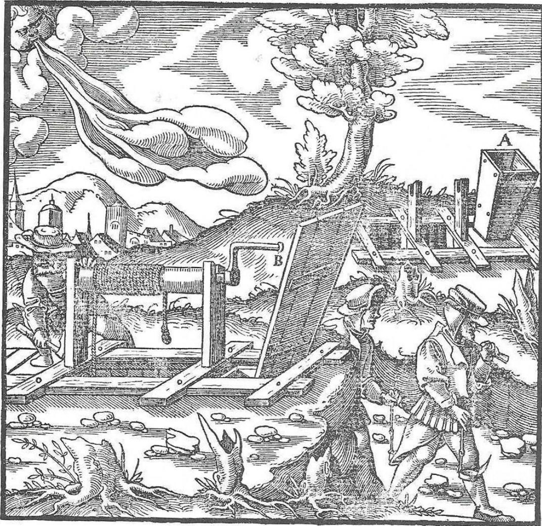
A—PROJECTING MOUTH OF CONDUIT. B—PLANKS FIXED TO THE MOUTH OF THE CONDUIT WHICH DOES NOT PROJECT.
