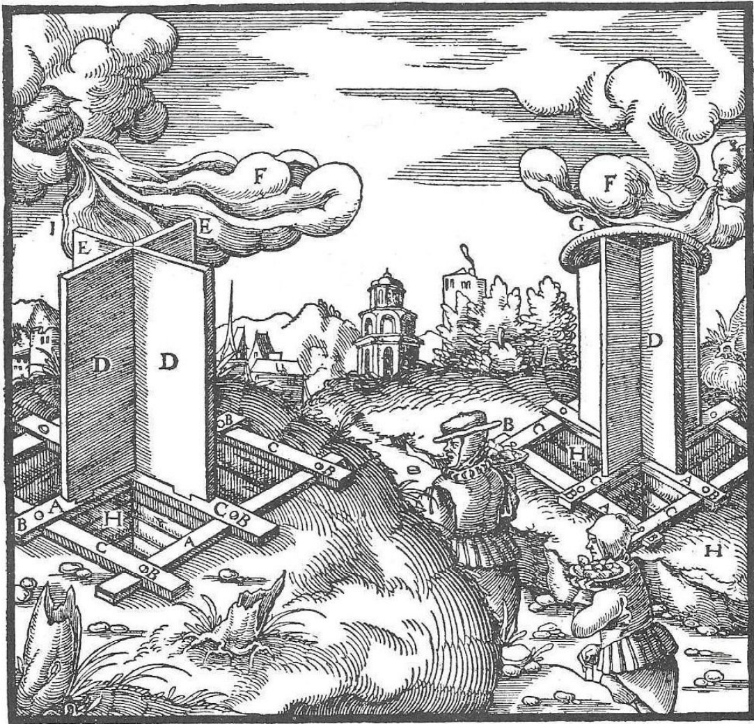
A—SILLS. B—POINTED STAKES. C—CROSS-BEAMS. D—UPRIGHT PLANKS. E—HOLLOWES. F—WINDS. G—COVERING DISC. H—SHAFTS. I—MACHINE WITHOUT A COVERING.
