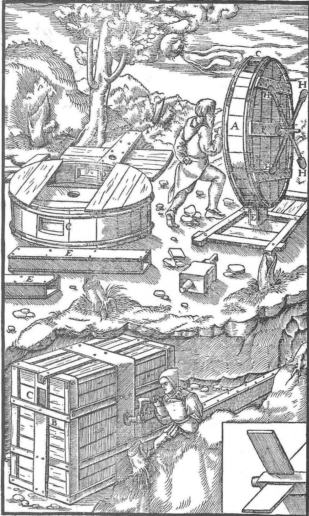
A—DRUM. B—BOX-SHAPED CASING. C—BLOW-HOLE. D—SECOND HOLE. E—CONDUIT. F—AXLE. G—LEVER OF AXLE. H—RODS.
